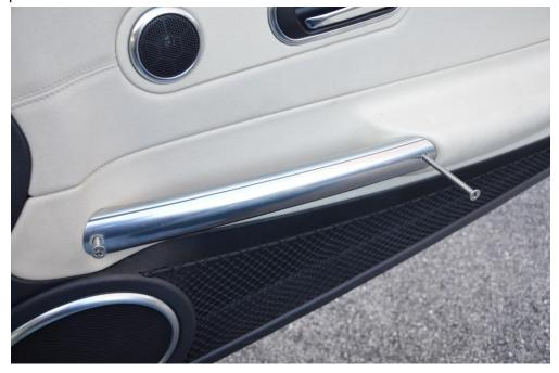
8. Tighten up with a Phillips screw driver evenly. In the passenger side case, I just had to tighten completely. On the driver's side since the broken pieces were now gone, I carefully, evenly tightened each end to make sure they were properly seated. Don't over-tighten since the bases are broken and removed and you will collapse the door panel and maybe also place the screws too deep and possibly cause internal damage.
