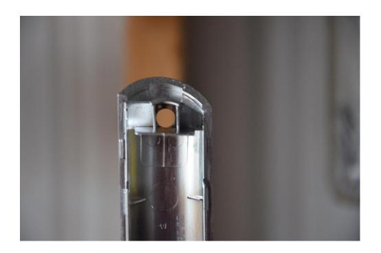
4. Once this is completed, you will need to countersink the other side so the screw is flush when installed. I did this by using a ½" drill bit IN MY HAND not in a drill. The plastic is very soft and will be destroyed if you use a drill. I carefully placed the ½" drill bit in the hole on the front side of the cover and turned it slowly to remove the plastic and create the countersink.
