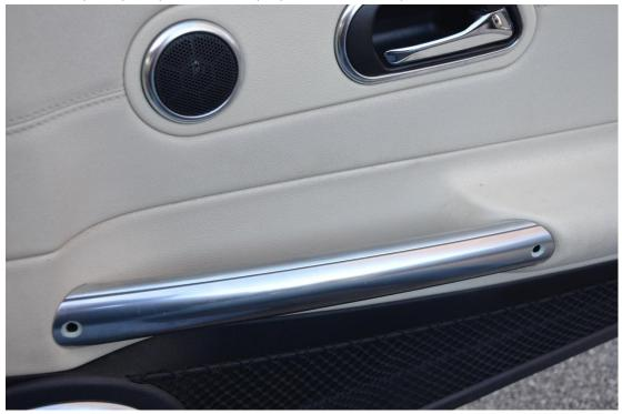
7. Insert screws and wiggle until you find the hole they need to be screwed back into in the door panel.
